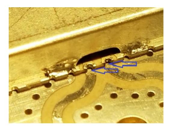
Another image to clearly show how the Splitter half-cut via circumferences align right to the edges of the Evaluation Board RF Traces:
