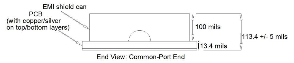
Mechanical Dimensions, Two-Port End View (board vias are not shown):
