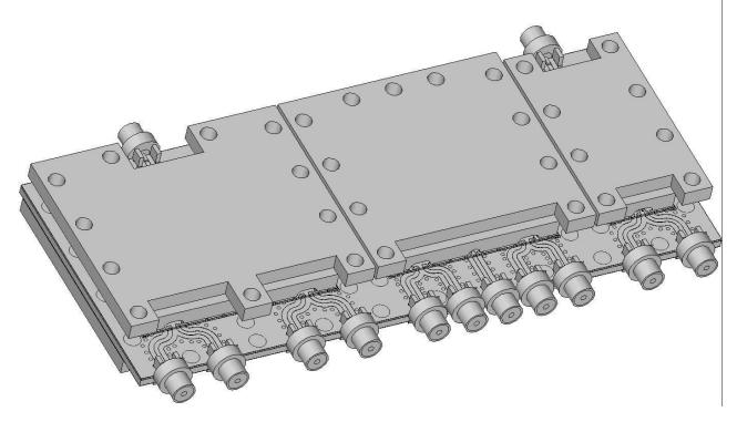
The "stiffener plates" do offer a significant level of heat-sinking since they are 93 mil thick Aluminum plates (one plate is placed in direct contact with the lid of the SMT splitter and the other plates is placed on the backside of the evaluation board...secured top to bottom with 2-56 screws/nuts). These plates are recommended for high power applications of BBTLine's Surface Mount Products.
